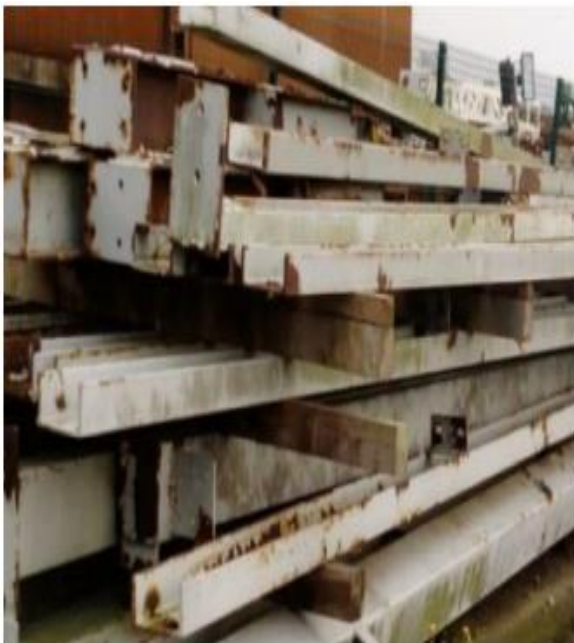
Fig.3. Steel from Demolished Building
