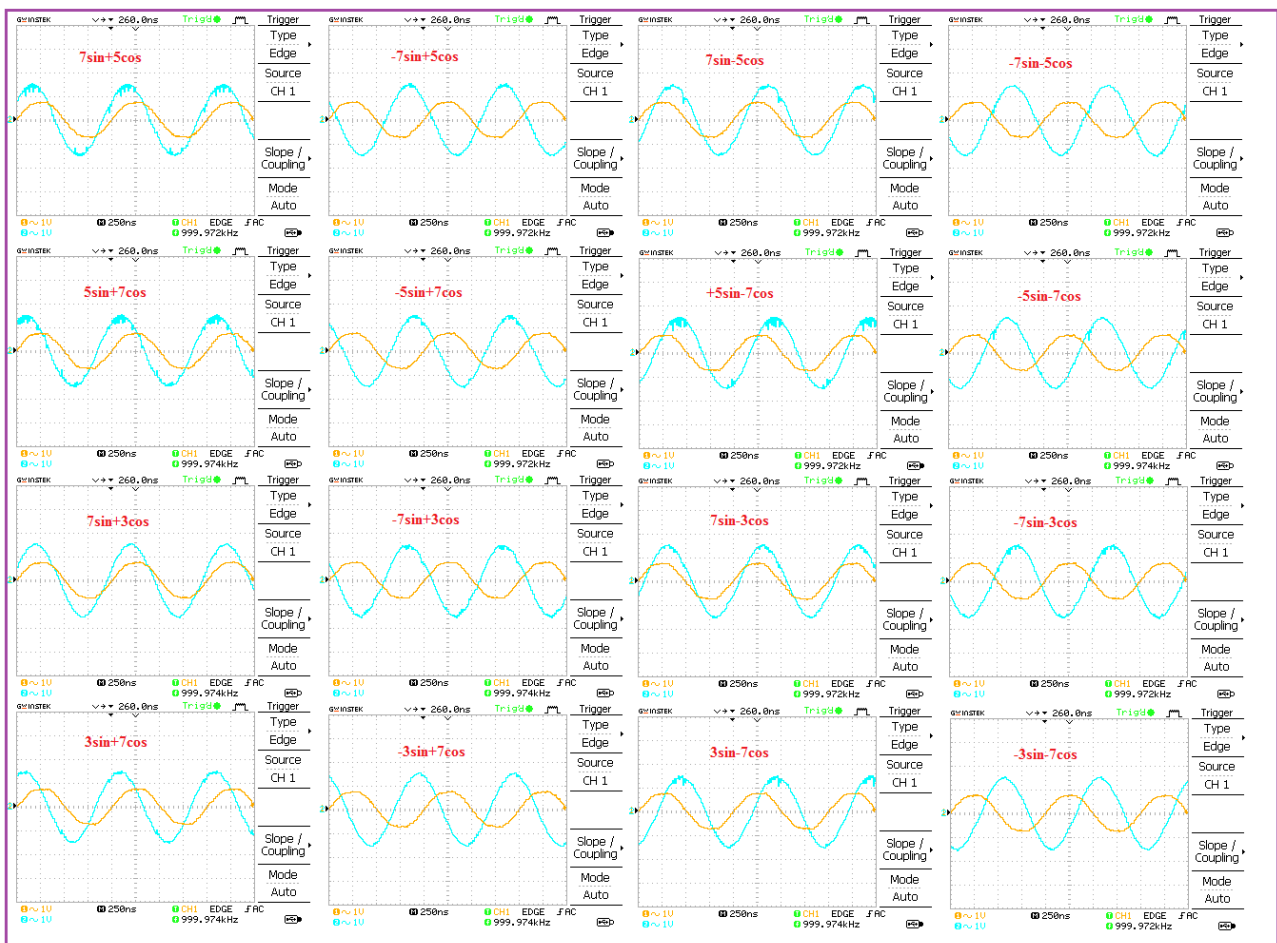
Figure (11-d) QAM-64 signals in time domain according values of table.2
